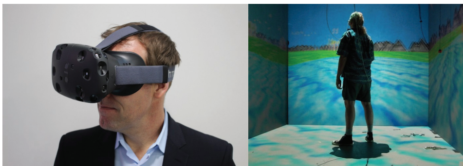
Figure 1. Virtual Reality Examples: (Left) HTC Vive headset that is tracked in 3D space (Vive.com 2018). (Right) A CAVE where the displayed image is projected onto a surrounding surface from the perspective of the user (Visibox.com 2018).
