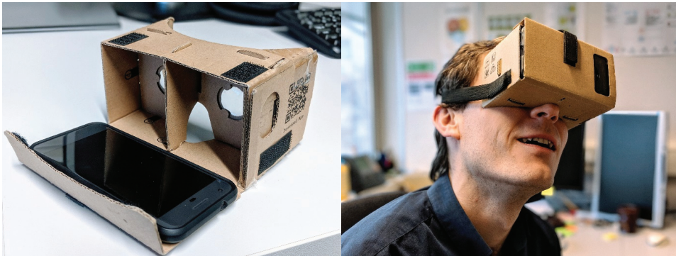
Figure 2. (Left) Shows how a mobile phone is placed as the display for Google Cardboard head-mounted display. (Right) Shows the placement of the Google Cardboard display in use.
